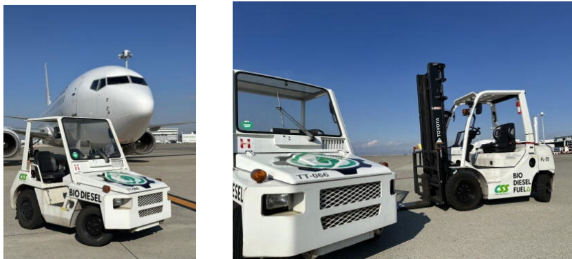
Figure 2-1-2 Towing tractor (left) and forklift (right) used in the demonstration experiment
